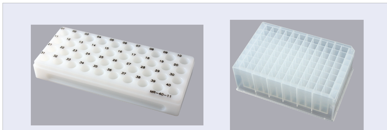
Figure 3. Available rack options - Left: 40-Position Micro Standards Rack; Right: 96-Well 2 mL Microtiter Plate Square Well.
