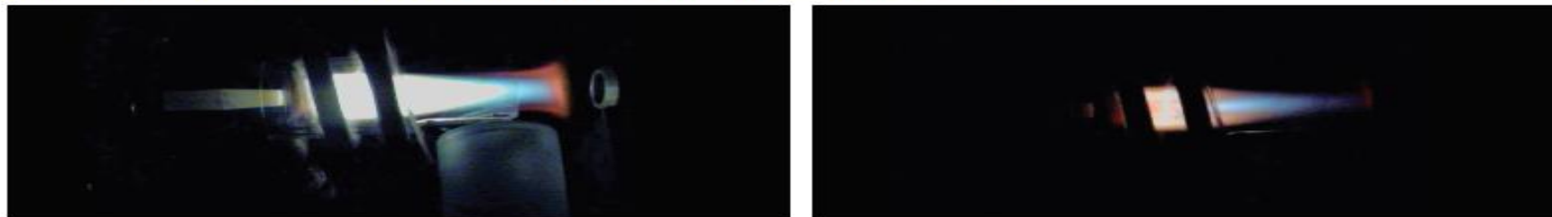
Figure 1. The figure on the left shows the angled base of the plasma which coincides with the angled shape of the load coil. The figure on the right shows the upward tilt of the axial channel and plasma tip as well as the differences in plasma density above and below the central channel.
