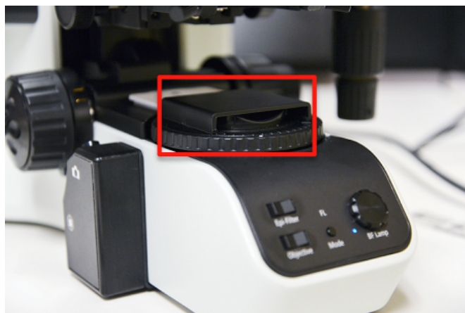
Figure 10. The Beam Block (the plastic cover shown in the red box) slides over the brightfield illuminator when you are using the Mantra system to take fluorescence image. The Mantra Snap program will prompt you to slide it into or out of place when necessary.
