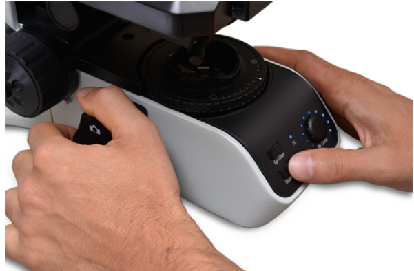
Figure 16. The Mantra 'Snap' button to take pictures is located on the handgrip on the left side of the Mantra instrument base. In the picture above, the Snap button is located under the user's left thumb. The Objective rocker switch to change objectives is located under the user's right thumb.
