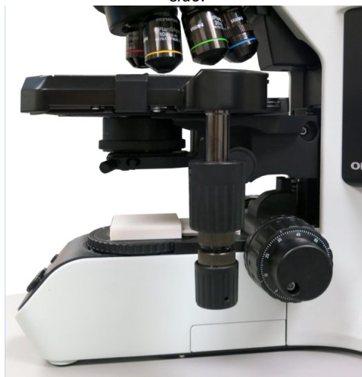
Figure 57. The right side of the Mantra instrument shown here with the knob for focus adjustment on the right. To the left of the knob are the stage controller knobs for X and Y axis control of the specimen under the objectives.
