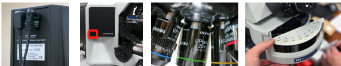
Figure 3. Power and USB cables plugged into the back of the Mantra imaging module (far left); the location of the Mantra Power switch outlined in red (middle left); objectives in their numbered turret positions (middle right); and epi-fluorescence filter cubes in their designated, numbered locations (far right).
