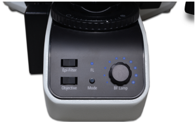
Figure 13. You can use the Objective rocker switch to select the objective you want. In brightfield mode, the blue light above the FL (fluorescence) label remains off and the Epi-Filter switch is deactivated. You can set the illumination level that is comfortable for you through the eyepieces using the BF Lamp knob on the right.
