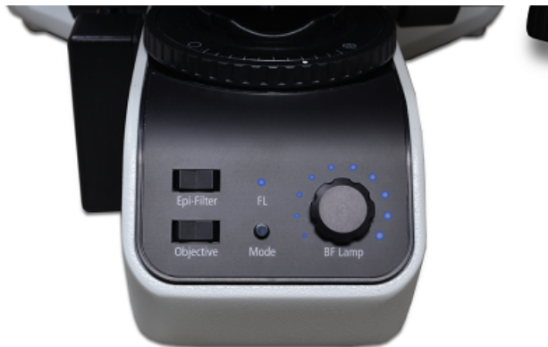
Figure 33. You can use the Epi-Filter rocker switch to select the epi-fluorescence filter that you wish to use, and the Objective rocker switch to select the objective you want to use. In fluorescence mode, the blue light above the FL (fluorescence) label is lit. The BF Lamp knob for setting the brightfield illumination level is deactivated when you are in fluorescence mode.
