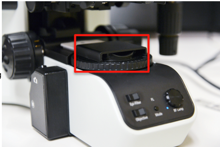
Figure 26. The Beam Block (the plastic cover shown in the red box) slides over the brightfield illuminator when you are using the Mantra system to take fluorescence image. The Mantra Snap program will prompt you to slide it into or out of place when necessary.
