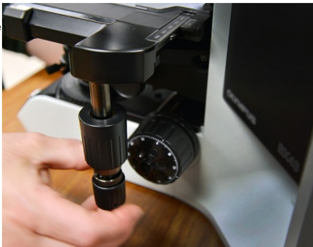
Figure 14. Use the Stage Control knob located by default on the right side of the Mantra instrument to move the microscope stage along the X- and Y-axes.
