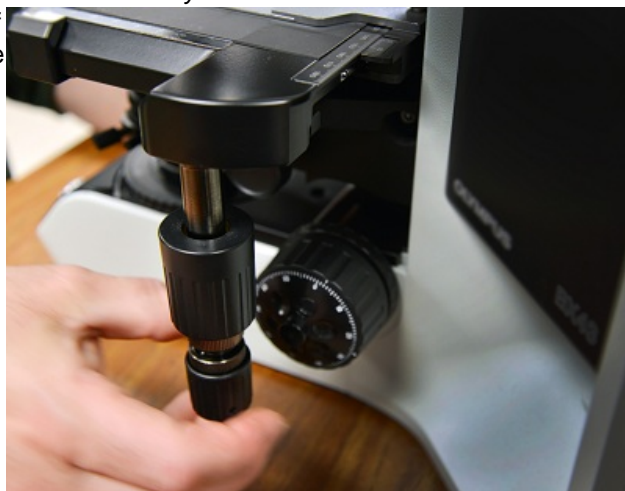
Figure 34. Use the Stage Control knob located by default on the right side of the Mantra instrument to move the microscope stage along the X- and Y-axes.
