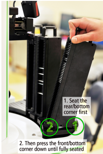
Figure 8. Mounting Slide Cassettes to the Slide Loader
