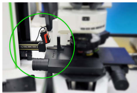
Figure 4. Loader Arm Facing the Stage
