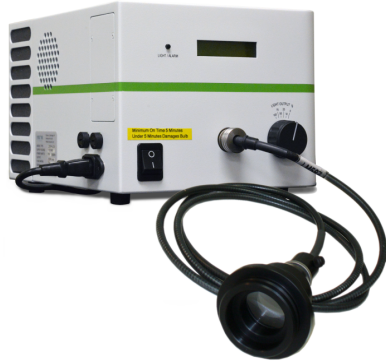
Figure 73. 200W Fluorescence Illuminator and liquid light guide with the collimator and adapter attached for the microscope.
