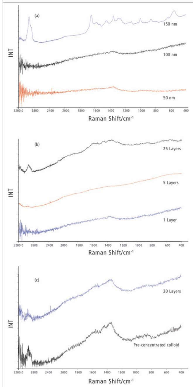
Figure 2. Effect of gold particle size and concentration on fingerprint spectra. (a) 50 nm and 100 nm dilute colloids and 150 nm Raman specification colloid, (b) single, 5 and 25 layers of 100 nm colloid and (c) x20 pre-concentrated 100 nm colloid compared to 20 successive layers of 100 nm colloid. Fingerprints were deposited on spotless MALDI inserts and the colloid deposited on top.
