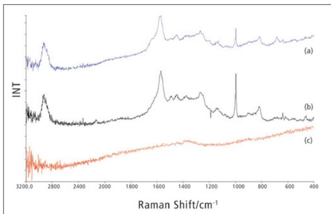
Figure 3. Spectra of (a) 100 nm dilute colloid, Na<sub>2</sub>SO<sub>4</sub> and fingerprint, (b) 100 nm dilute colloid and Na<sub>2</sub>SO<sub>4</sub> only and (c) 100 nm dilute colloid and fingerprint only.
