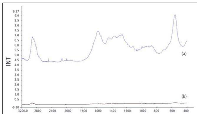
Figure 4. Effect of deposition sequence on fingermark spectra using 150 nm Raman specification gold colloid. (a) colloid deposited before fingermark and (b) fingermark deposited before colloid.
